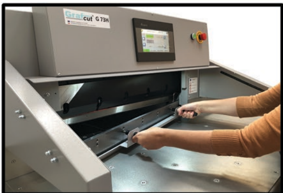
Safe Blade Change Procedure with Cradle
