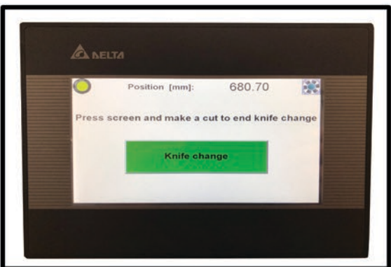
Knife Change Mode for Safe Blade Changes
