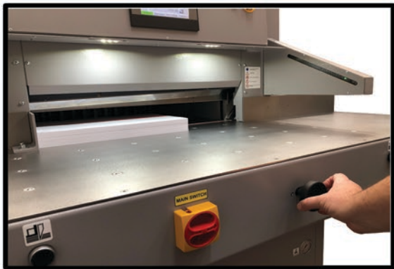
Push & Lock Fine Adjust Dial for Perfect Postioning
