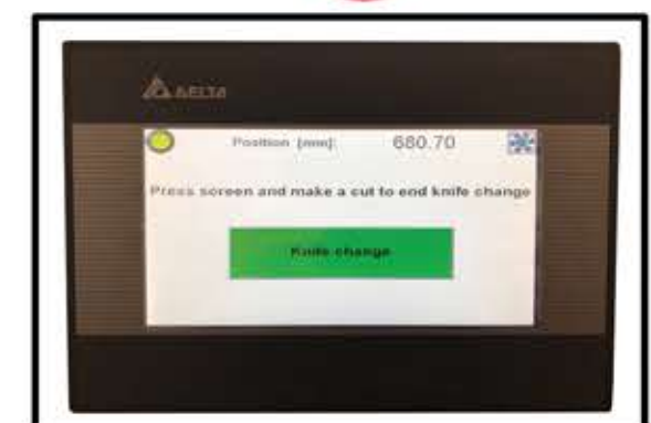
Knife Change Mode for Safe Blade Changes
