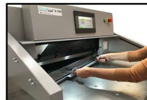
Safe Blade Change Procedure with Cradle
