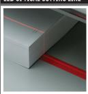
The optical cutting line indicator with especially bright and durable LEDs guarantees easy alignment of cutting marks for precise cuts.
